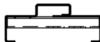
Befestigung Hutanker S2+TZ fissaggio staffa ad "U" S2+TZ fitting with "U" bracket S2+TZ
