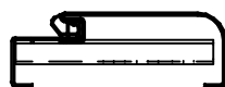
Befestigung Hutanker S2+TZ fissaggio staffa ad "U" S2+TZ fitting with "U" bracket S2+TZ
